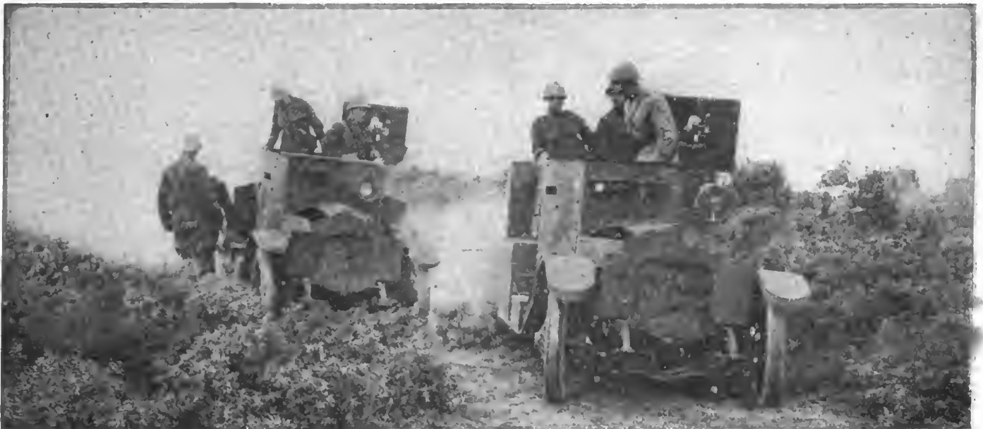
Two of the Belgian armored cars on skirmish work. Note the single large headlight and how the armor plate protects the engine hood and radiator. The motorcycle men are between the cars and the enemy so the crews are simply awaiting the word to advance
